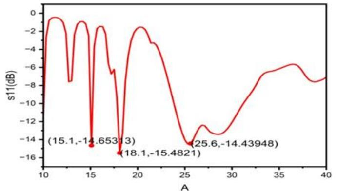
Fig.2. Antenna return loss (S11)
