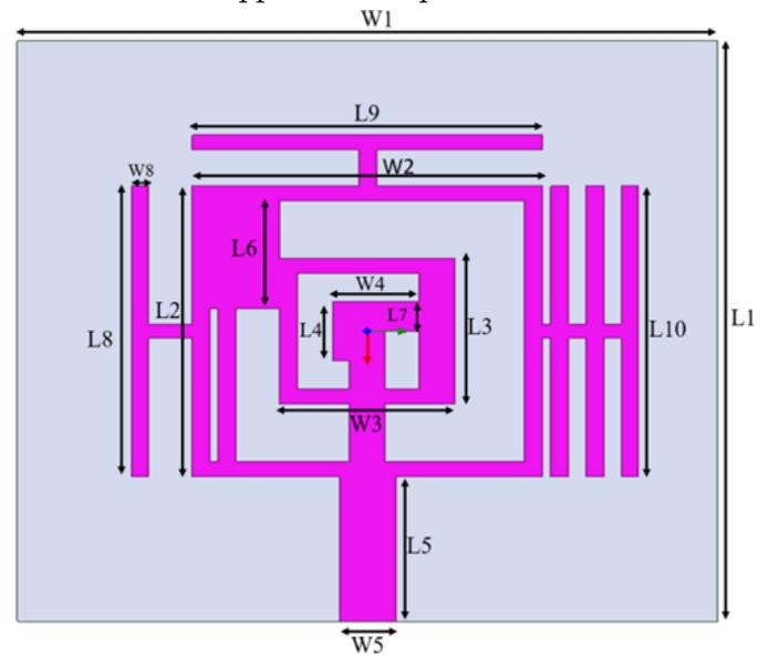
Fig 1.A. Antenna Design Structure with dimensions
