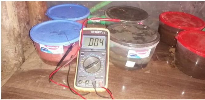
Figure 2 : Set-up of H-shaped microbial fuel cells with a multi-meter
