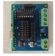
provide, you need some kind of switch that takes a small current, amplifies it, and produces a larger current that still drives the motor. This whole process is carried out by the so-called engine controller. With the L293D motor driver IC, this task is easy and has served many applications with relative ease.
