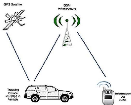
The vehicle owner receives the SMS that his vehicle is stolen. Then he can send back an SMS to the GSM modern to step the engine. Here, GSM Modern is interfaced to the PIC microcontroller that receives the message, the O/P of which activities a mechanism
