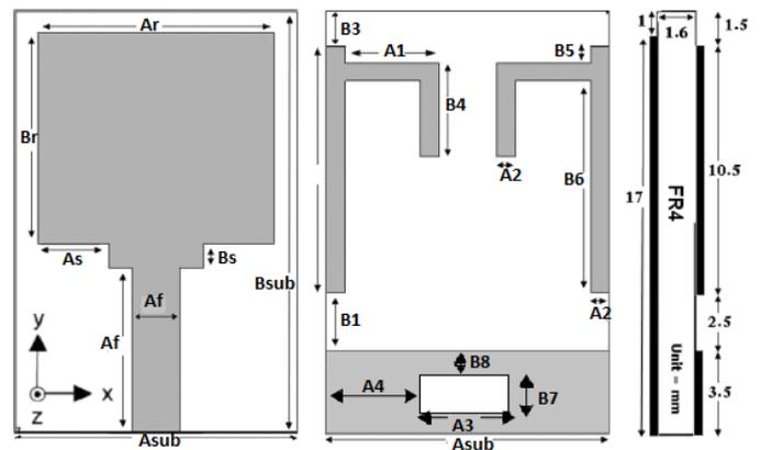
**Figure 1.** Geometry of proposed antenna in millimeters
