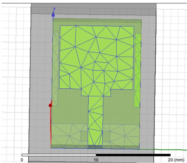
**Figure 5.** Mesh analysis plot
