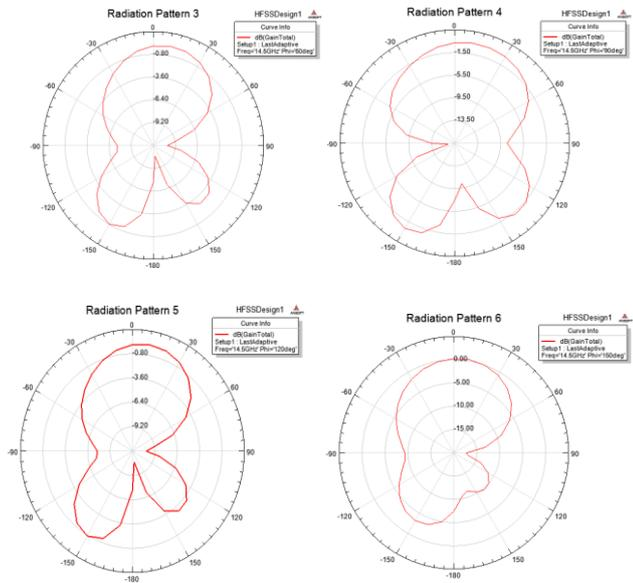
**Figure 4a.** Radiation patterns at different angles
