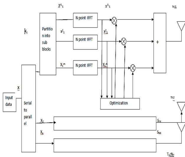
fig:the block diagram of PTS scheme in MIMO-OFDM
