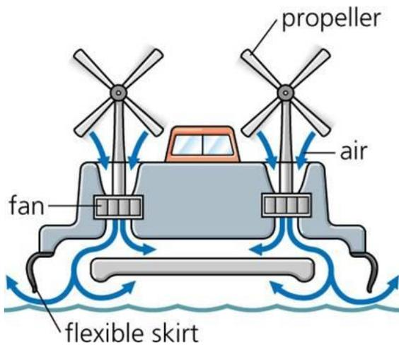
**Figure 1.** Schematic diagram
