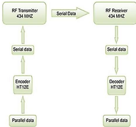
Figure 4. Transmission Diagram
