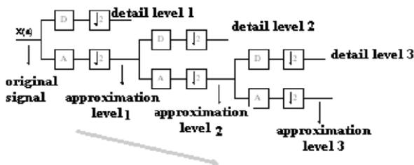
**Figure 1.** Decomposition scheme Mallat's algorithm
