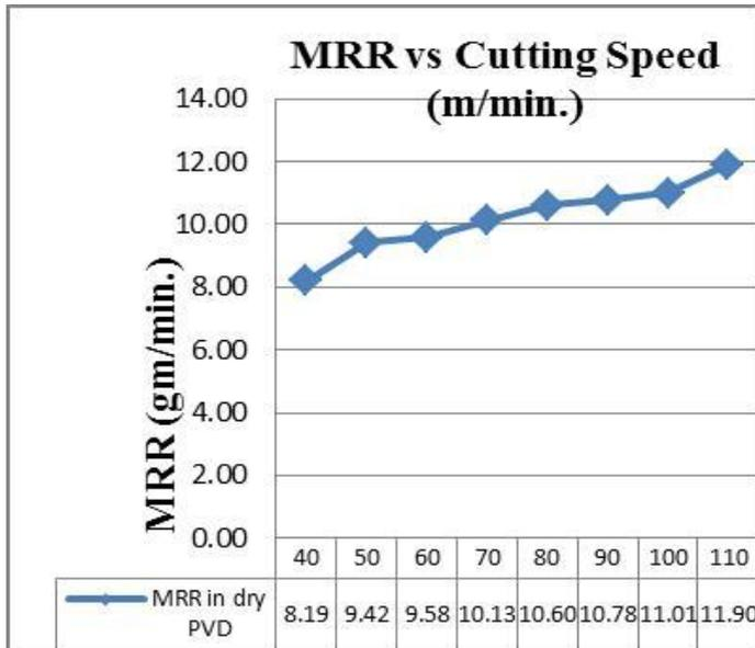
**Figure 1.** Effect of varying cutting speed on MRR
