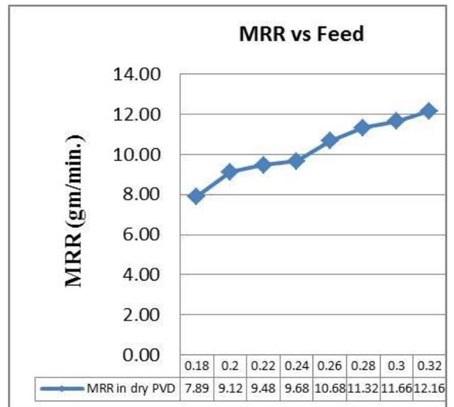
**Figure 2.** Effect of varying feed on MRR
