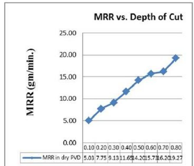
**Figure 3(1).** Effect of varying depth of cut on MRR
