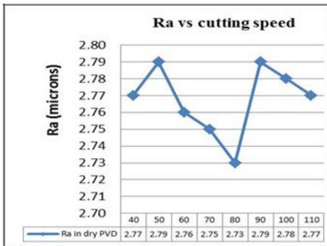
Figure 4(2). Effect of cutting speed on Ra
