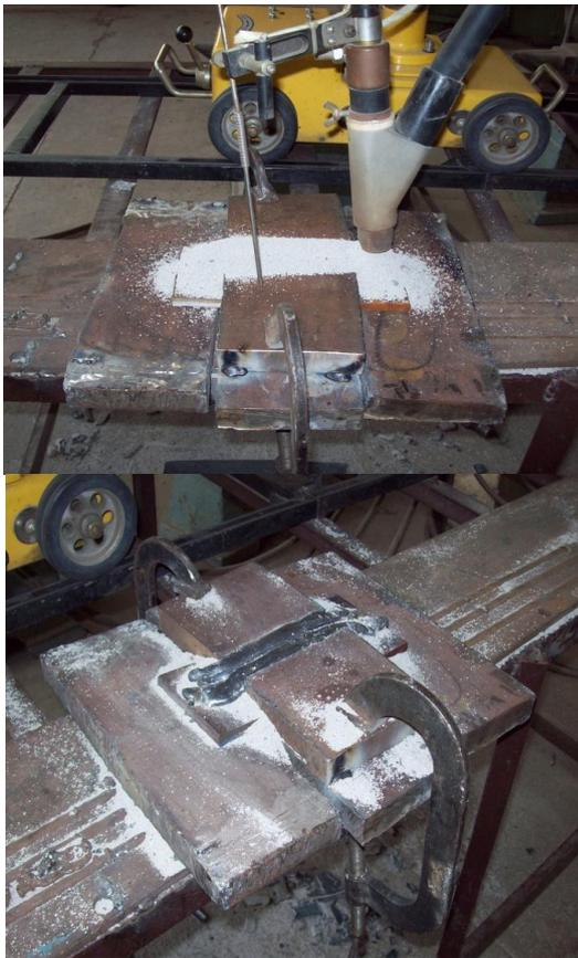
shape. As the stress approaches that of the tensile strength, a material that has begun to flow forms a narrow, constricted region that is easily fractured. Tensile strengths are measured in units of force per unit area. Welded specimen made from base metal and fined the tensile strength and stress-strain curves.
