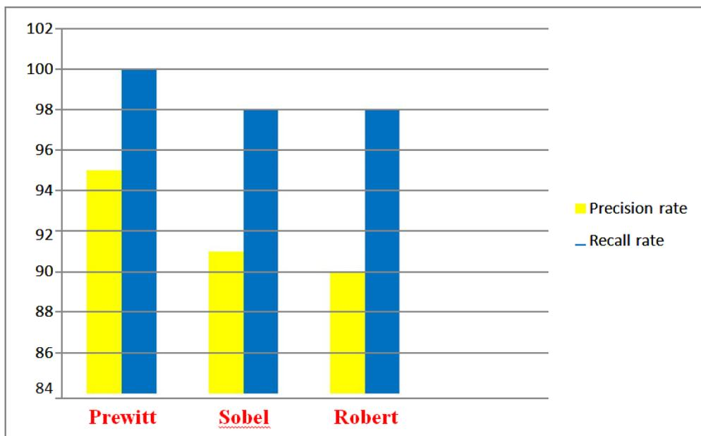
From the above graph it is cleared that precision rate and recall rate using prewitt edge detection is high compared with sobel and Robert edge detection method.
