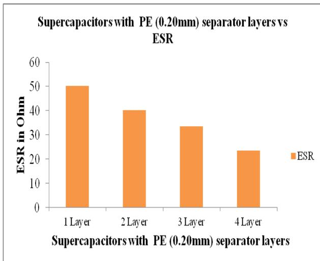
**Figure 7:** ESR of PE (0.20mm) separator layers of supercapacitor
