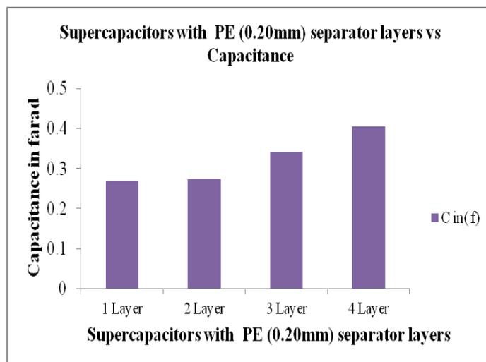
**Figure 6 :** Capacitance of PE (0.20mm) separator layers of supercapacitor
