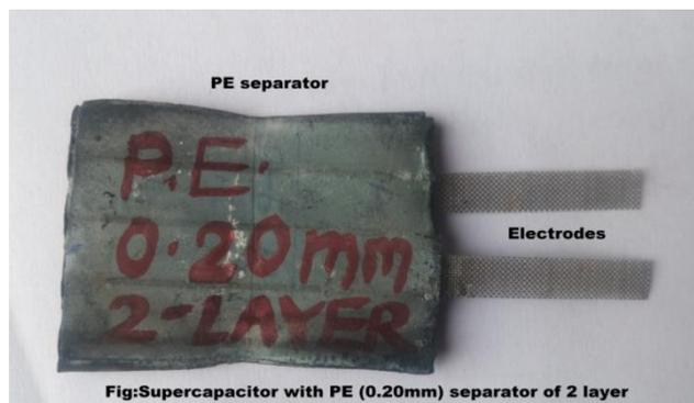
Figure 1: PE (0.20mm) separator two layers of super capacitor
