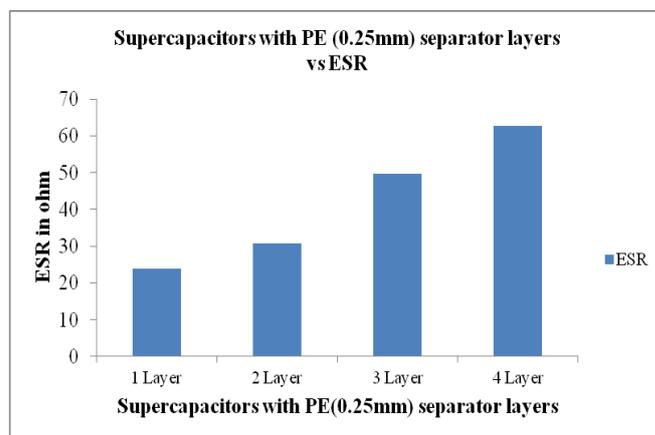
**Figure 5:** ESR of PE (0.25mm) separator layers of supercapacitor
