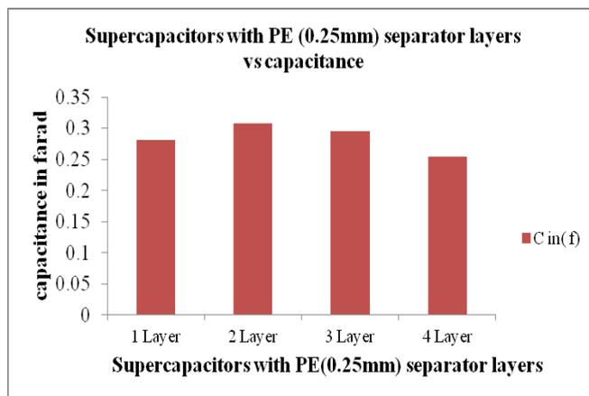
**Figure 4 :** Capacitance of PE (0.25mm) separator layers of supercapacitor
