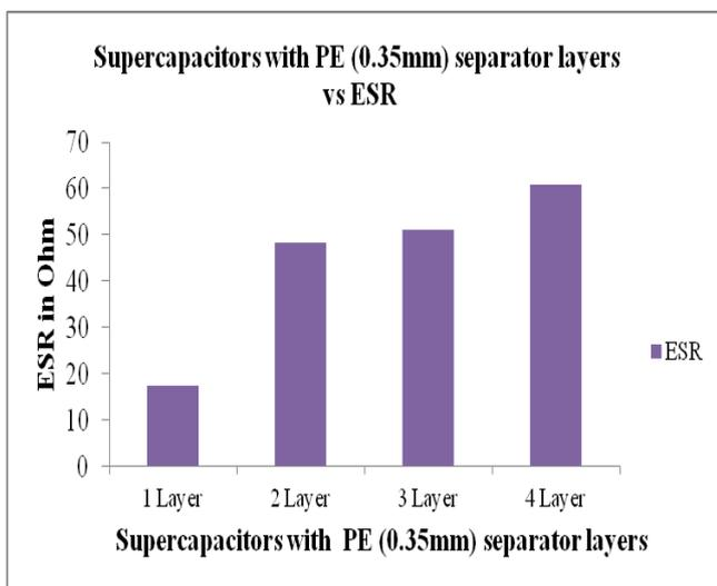
**Figure 3:** ESR of PE (0.35mm) separator layers of supercapacitor
