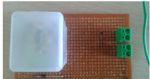
Figure 11. Relay switching unit (to switch the connection from parallel to series and vice versa).
