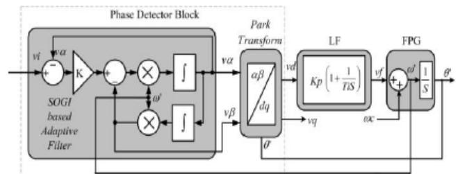
Figure 3. SOGI-QSG & Parks Transform based Phase Detector.
