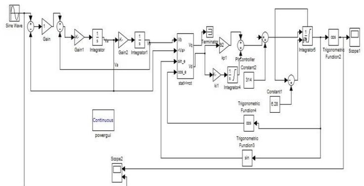
Figure 5. Simulation of SOGI PLL
