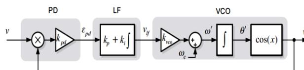
Figure1. Structure of basic PLL
