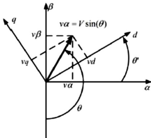
Figure 4. Vector diagram of SOGI-PARK based Phase detector
