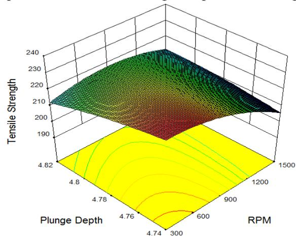
**Figure 6:** Interaction effect of tool rotational speed and plunge depth on tensile strength
