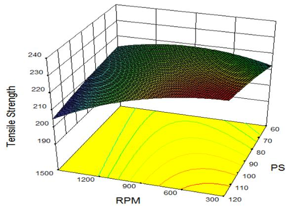
**Figure 5:** Interaction effect of tool rotational speed and processing speed on tensile strength
