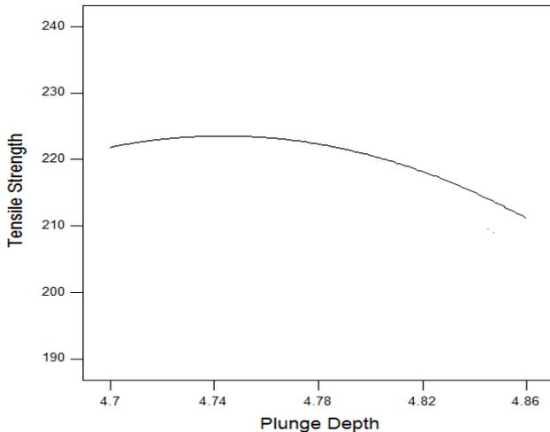
**Figure 4:** Direct effect of plunge depth on tensile strength
