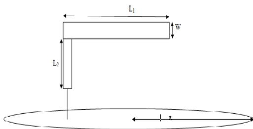
**Figure 1.** The structure of a PILA with a finite ground plane
