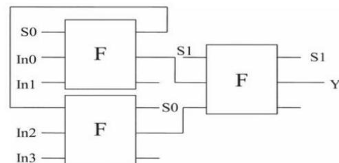
Figure 6: Fredkin Gate based reversible 4:1 MUX
