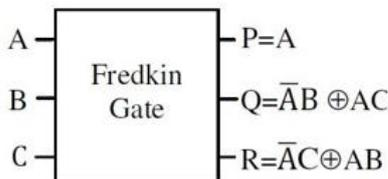
Figure 4: Block Diagram of Fredkin Gate
