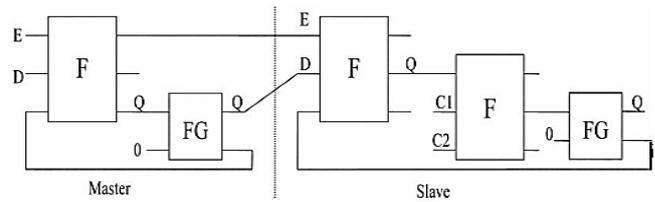
Figure 5: Fredkin Gate based Reversible D flip flop
