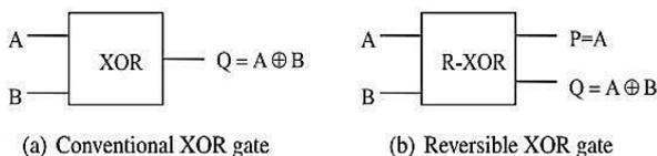
**Figure 1:** Block Diagram of Conventional Gate and Reversible Gate
