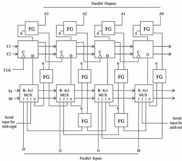
**Figure 6:** 4-Bit Reversible Universal Shift Register
