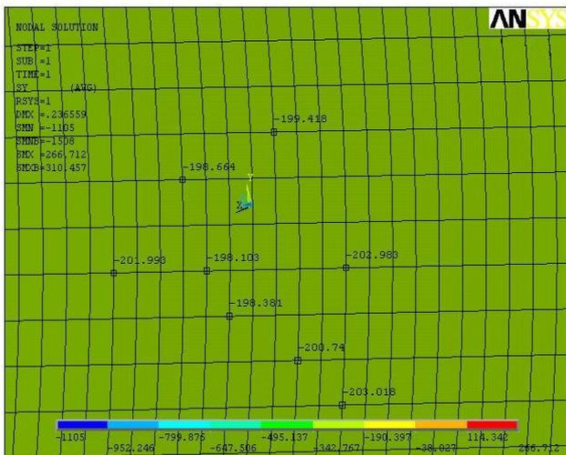
Figure 4(e) :Max .thermal stress on Different Nodes of inside surface
