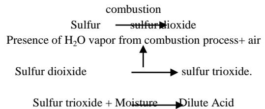
Result of all above reaction formation of dilute acid and its precipitation. This affects the surface of liner undergoes to a rapid corrosive attack. And the results effects on performance of cylinder liner in internal combustion engine.
