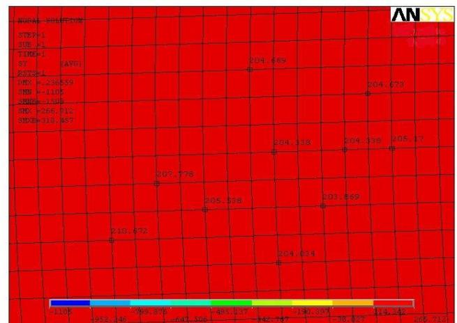
**Figure 4(d) :** Max thermal stress on Different Nodes of outside surface
