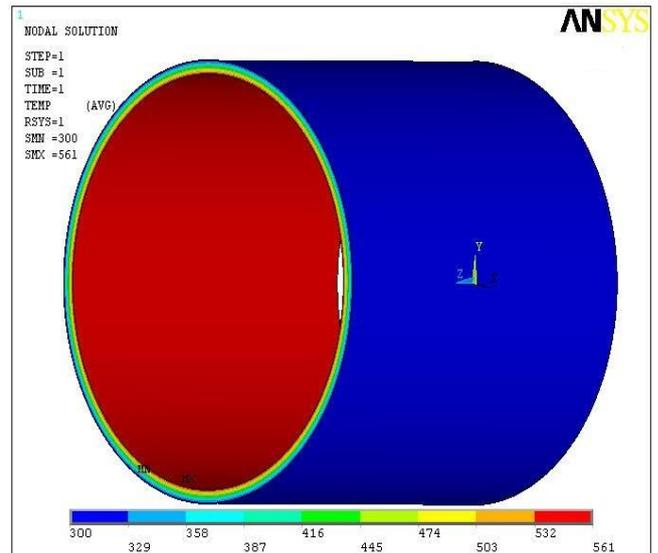
**Figure 4(c):** Temperature distribution along the thickness of liner is shown in the Nodal Solution
