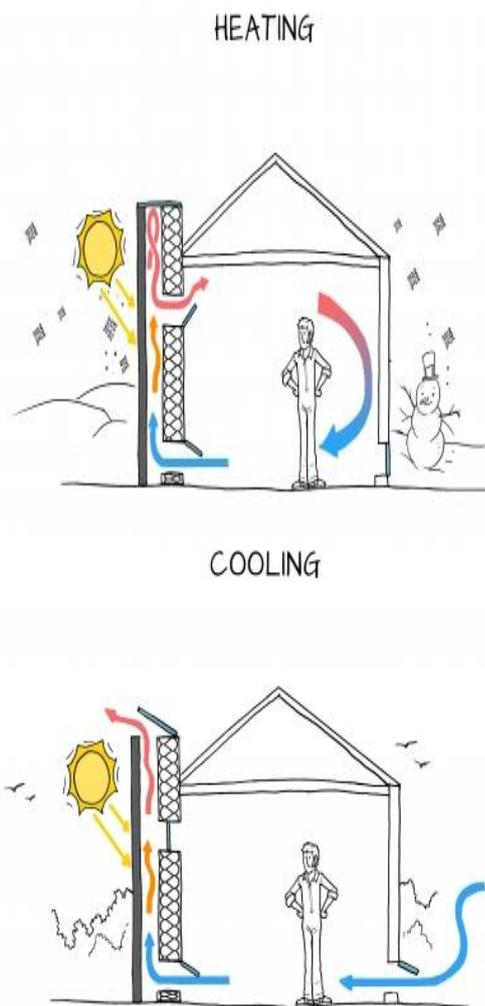
**Figure 3.** The effect of opening or closing of the stack or chimney <sup>[1]</sup>
