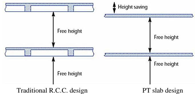
**Figure 1:** Height comparison of R.C.C. & PT slab design [3]
