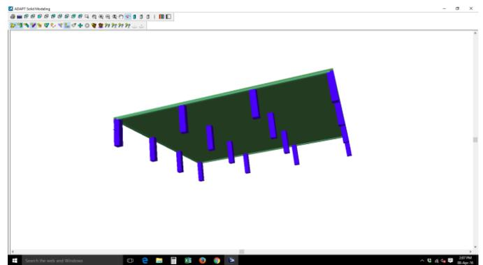
Figure 4: The typical view of the (7x7) m panel in Adapt
