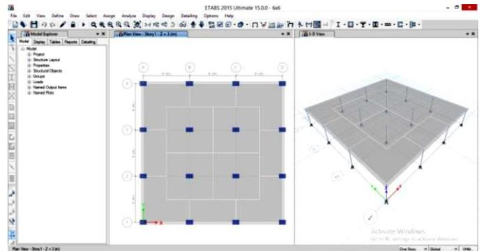
Figure 3: The typical view of the (7x7) m panel in Etabs
