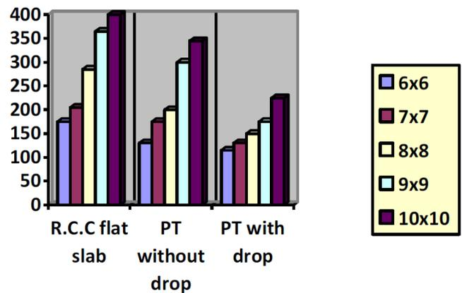
**Figure 5.** Thickness comparison bar chart for each panel size
