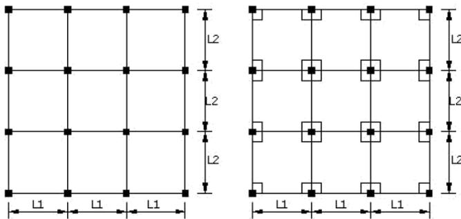
Figure 2: Plan of slab with drop and without drop
