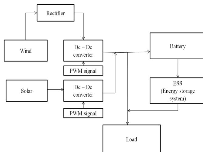
**Figure 1.** Block Diagram of Proposed Design
