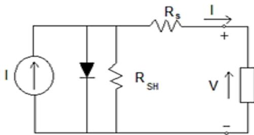
**Figure 3.** Single diode module of a PV Cell
