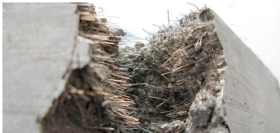
Figure 1. Fracture of SFRC [SIKA.COM]
