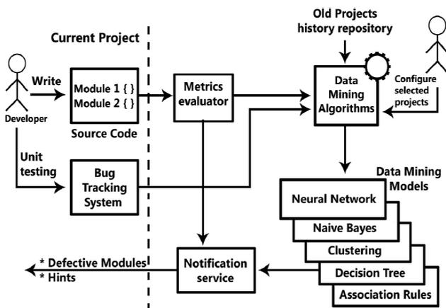
Figure 1. Architecture for defective module identification using data mining and Software metrics<sup>[2]</sup>
