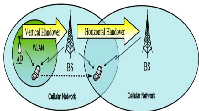
Figure 1. Procedure of Vertical Handoff [2]
