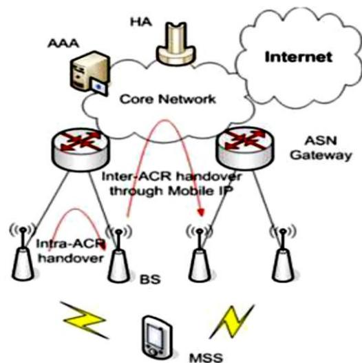
Figure 2. Network Architecture of Mobile WiMAX [4]
