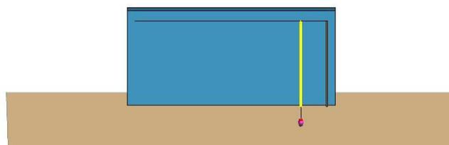
Figure 2. (b) Inverted-F antenna structure
