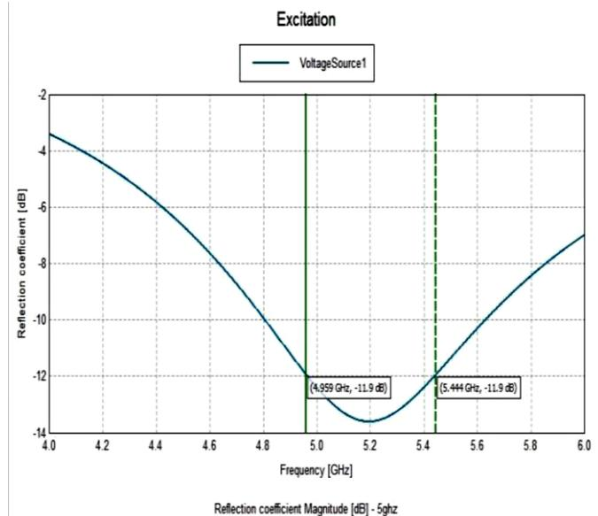
Figure 3. (c) S-parameter of monopole antenna
