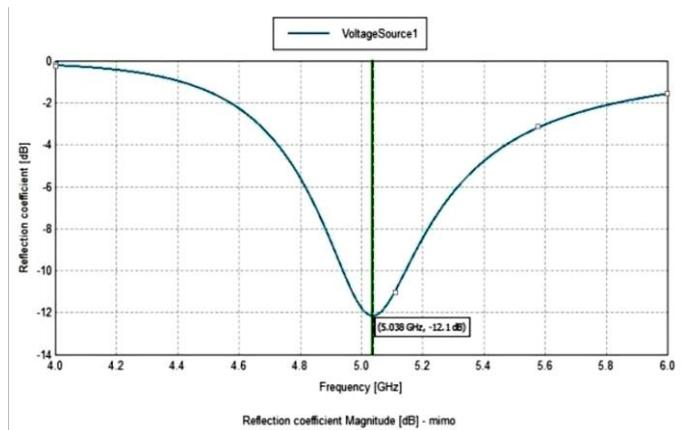
**Figure 3.(h)** Sparameter of MIMO antenna
