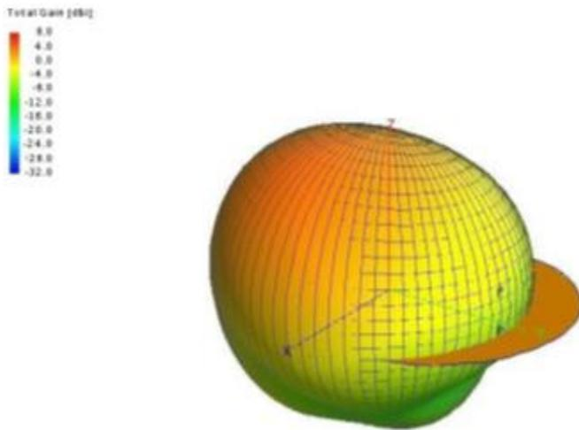
**Figure 3. (i)** Gain of MIMO antenna
