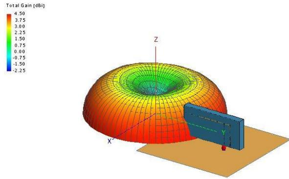
**Figure 3. (f)** Gain of inverted-F antenna
