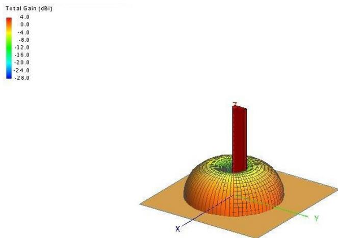
**Figure 3. (e)** Gain of Monopole antenna
