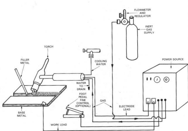
**Figure 1.** Schematic Illustration of PCTIG welding
