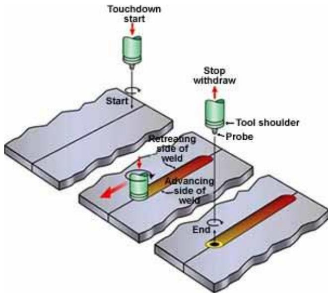
**Figure 1.** Friction Stir Welding
