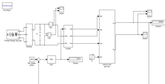
Figure 4. Closed loop control with PI controller ( module model )
