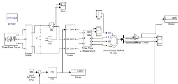
Figure 3. Closed loop control with PI controller (Readymade module )
