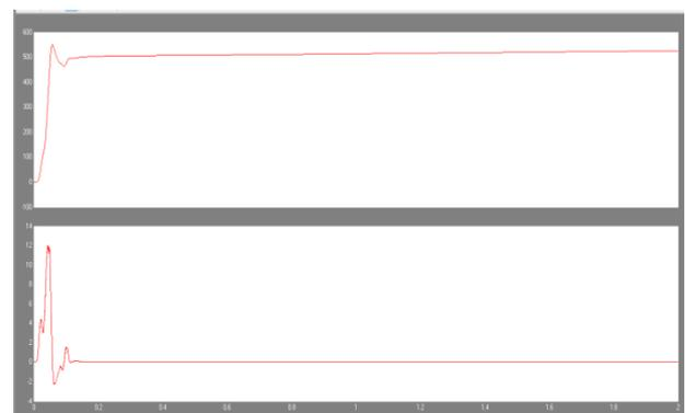
Figure 8. Speed and Torque of I.M with PI controller with Module Model (Base speed 500 RPM)
