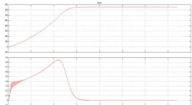
**Figure 6.** Speed and Torque of I.M with Module Model
