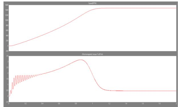
**Figure 5.** Speed and Torque of I.M with Readymade Model
