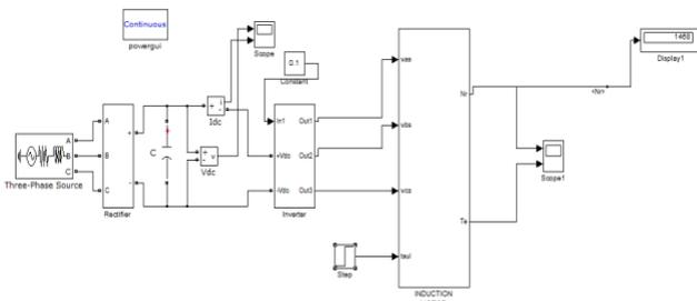
**Figure 2.** Open loop with module model of I.M
