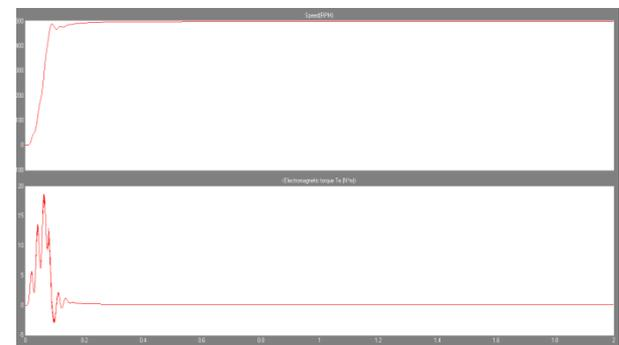
Figure 7. Speed and Torque of I.M with PI controller With Readymade Model (Base speed 500 RPM)
