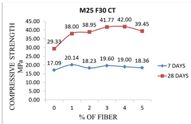
Figure 3: Comparison between 7 & 28-days compressive strength (MPa) for M25 F30
