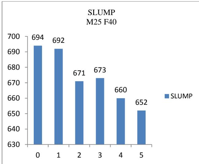
Figure 1: Slump Test M25 F40
