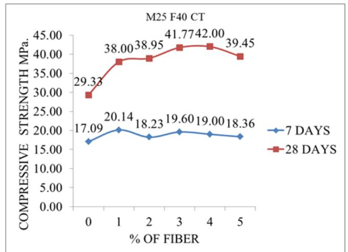
Figure 5: Comparison between 7 & 28-days compressive strength (MPa) for M25 F40
