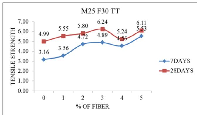
**Figure 6:** Comparison between 7 & 28-days tensile strength (MPa) for M25 F30
