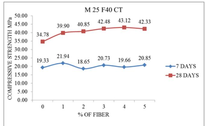
Figure 4: Comparison between 7 & 28-days compressive strength (MPa) for M25 F40
