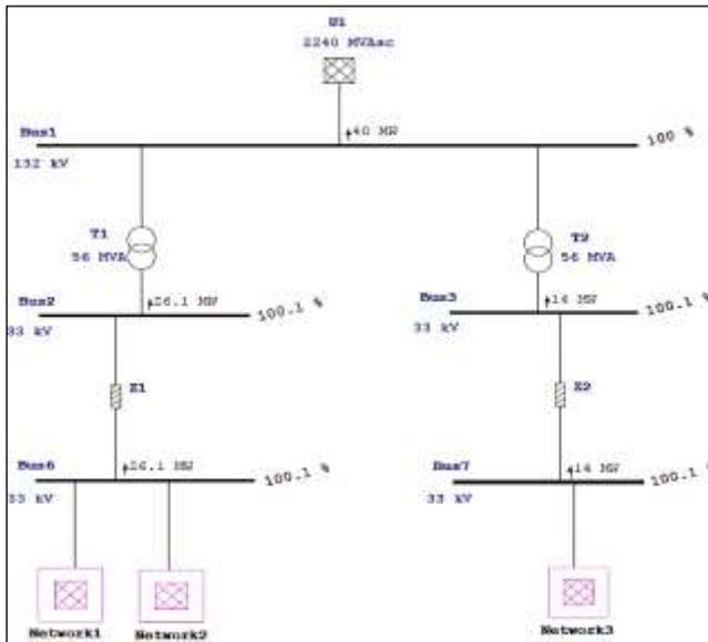
**Figure 3:** Load Flow Analysis
