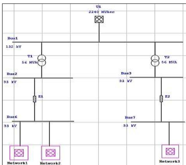
Figure 1. Layout of the Wind Farm
