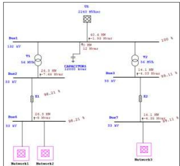
**Figure 7:** Reactive Power Analysis with Compensation
