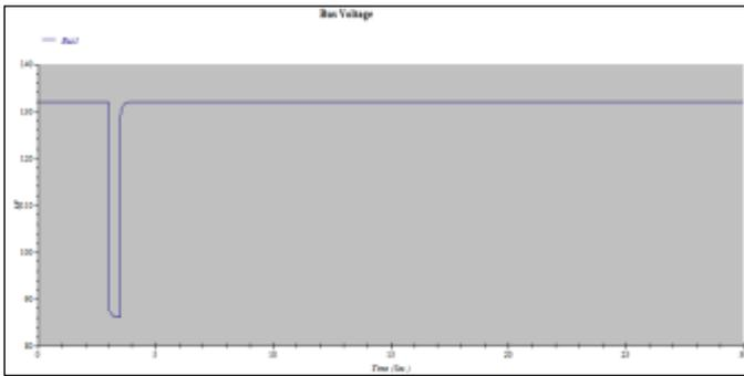
**Figure 5:** Voltage at Bus 1 during Single L-G fault
