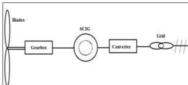
Figure 2. Block diagram of SCIG based WECS
