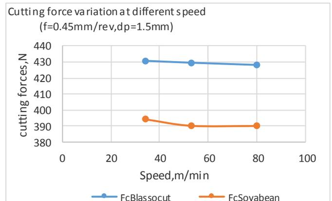
**Figure 3.** Variation of Cutting Forces With Respect To Speed
