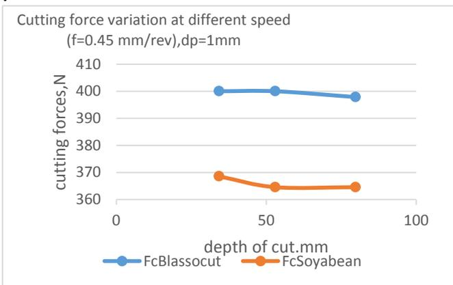
**Figure 2.** Variation of Cutting Forces With Respect To Depth of Cut
