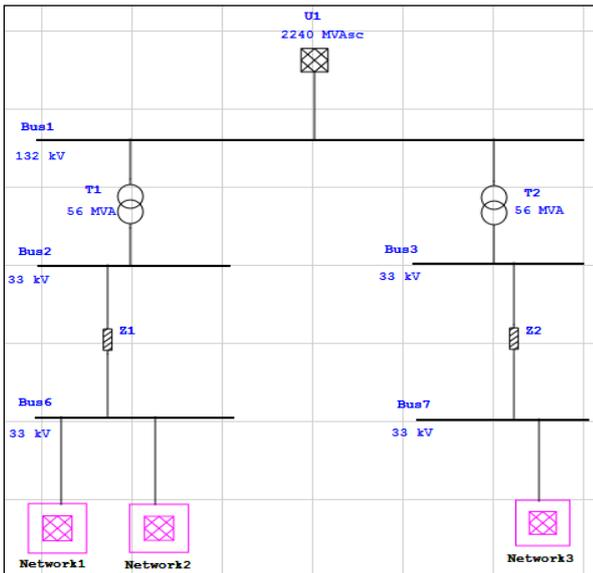
**Figure 1.** Single line diagram of the Wind Farm
