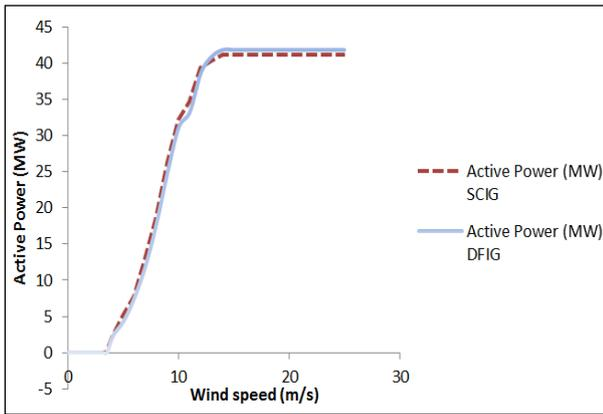
**Figure 6.** Active power curve comparison of SCIG and DFIG
