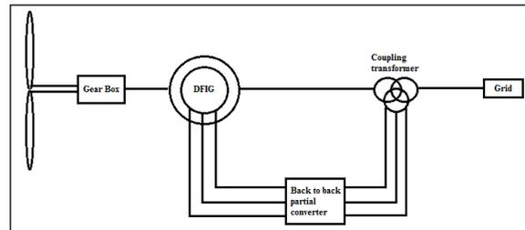
**Figure 3.** Block diagram of DFIG
