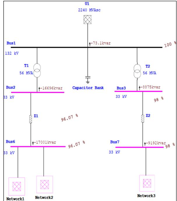
**Figure 8.** Reactive power compensation with capacitor bank
