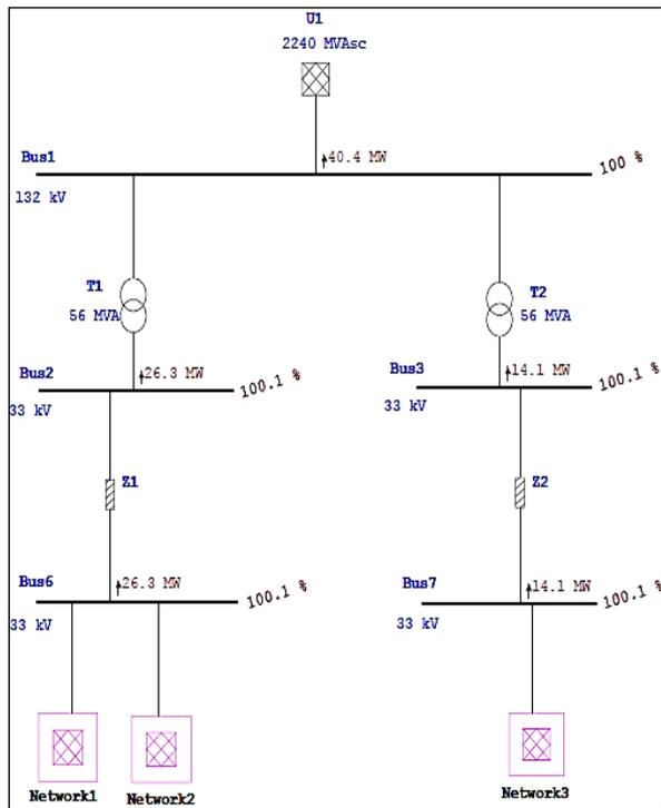
Figure 5. Active power flow for DFIG at nominal speed
