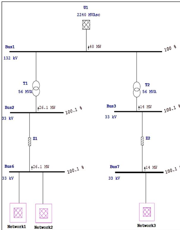
Figure 4. Active power flow for SCIG at nominal speed
