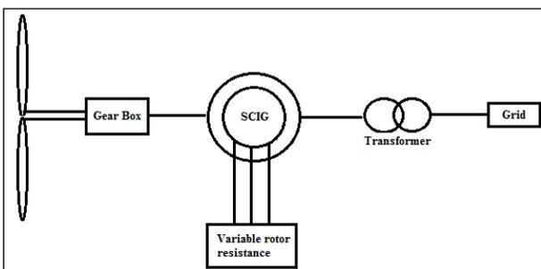
**Figure 2.** Block diagram of SCIG
