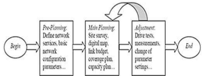
Figure 1. Radio Network Planning Process
