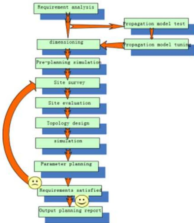
**Figure 2.** Flow Diagram for Network Planning
