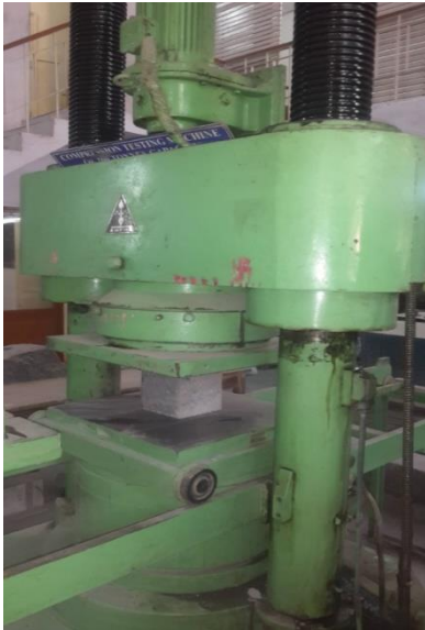
Figure 3. Experimental setup of compression test
