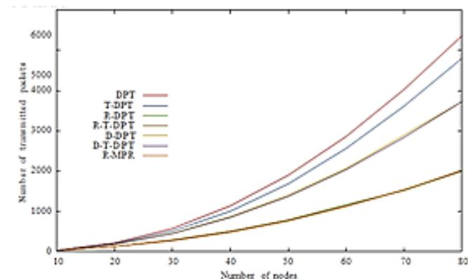
**Figure 4.** Proposed approaches compared to best existing ones. We observe that (i) random network coding still outperforms deterministic one and that (ii) using network coding reduces the gap between tree-based techniques.
