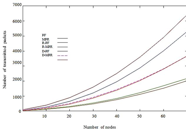
**Figure 2.** Comparison of existing solutions for OLSR. Observe how random network coding performs better than the deterministic one, whatever the technique it is associated to.
