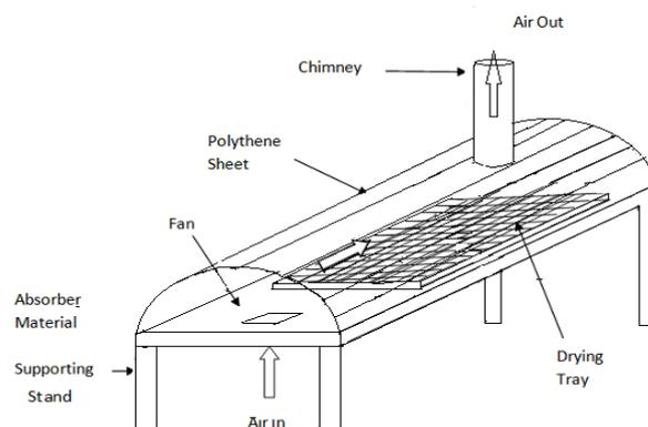
Figure 1. Schematic of Solar Tunnel Dryer
