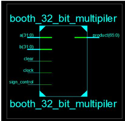
Figure 7. RTL Schematic of 32-bit Booth multiplier.
