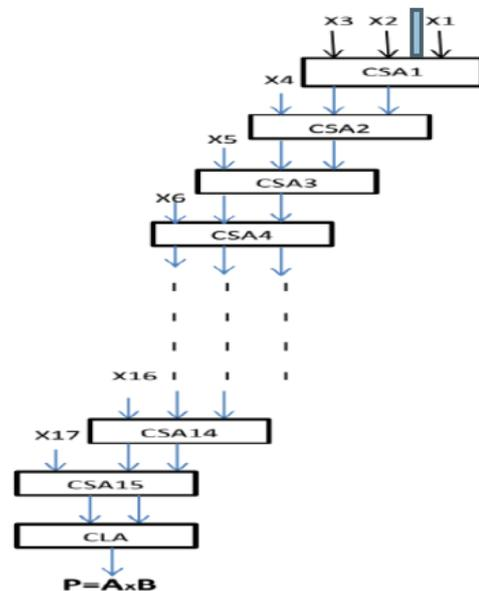
Figure 6. Partial product adder logic
