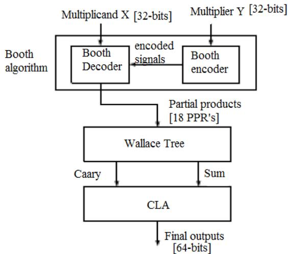
**Figure 2.** Architecture of the 32-bit Booth Encoder Multiplier
