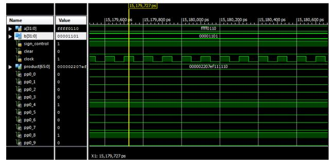
Figure 10. 32-bit signed by unsigned numbers multiplication in Hexadecimal representation
