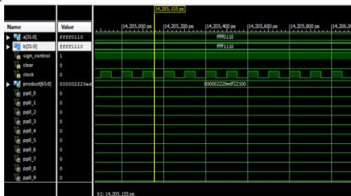
Figure 9. 32-bit signed number multiplication in Hexadecimal representation
