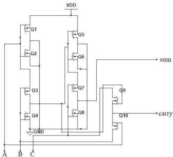
**Figure 5.** Schematic for SERF Adder
