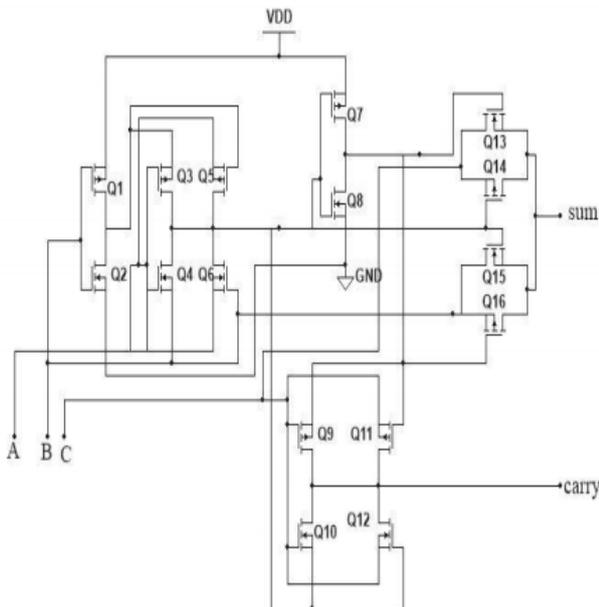
**Figure 11.** Hybrid Adder Circuit Design
