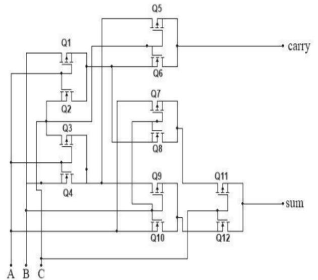
**Figure 8.** Multiplexer based Adder circuit design
