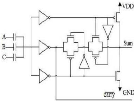
**Figure 10.** Inverter and Transmission Gate based adder design
