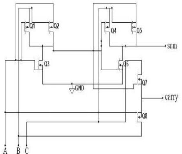
**Figure 9.** 8T Adder circuit design
