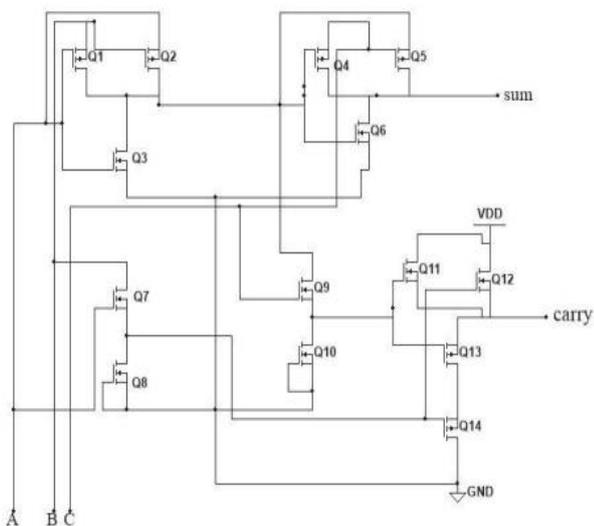
**Figure 6.** 14T transistor Adder circuit
