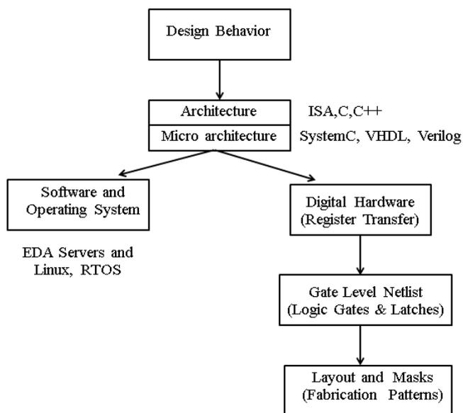
**Figure 3.** Design representation levels and formats associated
