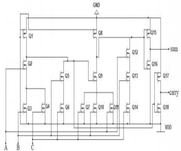
**Figure 7.** Pseudo nMOS Adder Circuit
