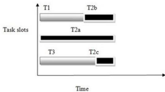
**Figure 5.** Mitigation of the straggler using SkewTune
