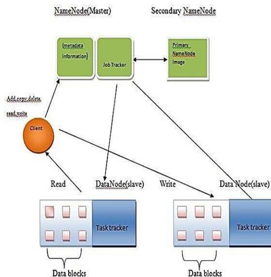
Figure 1. Block diagram of HDFS architecture
