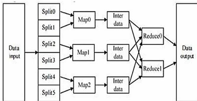
**Figure 2.** Working process of MapReduce
