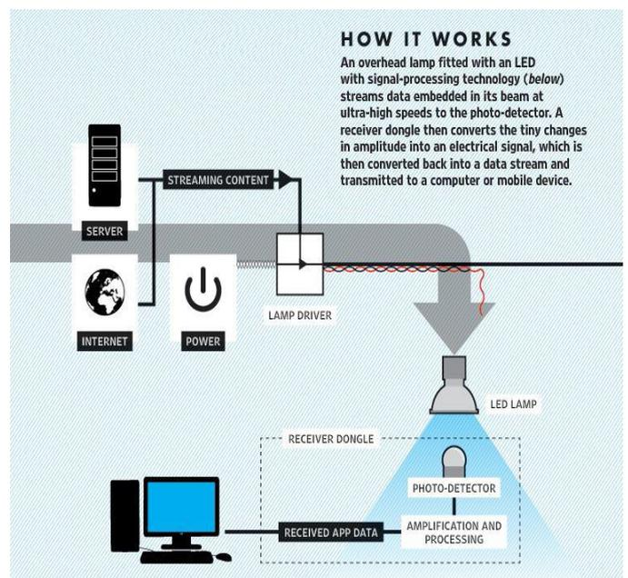
To further get a grasp of Li-Fi consider an IR remote. It sends a single data stream of bits at the rate of 10,000-20,000 bps. Now replace the IR LED with a Light Box containing a large LED array. This system is capable of sending thousands of such streams at very fast rate.
