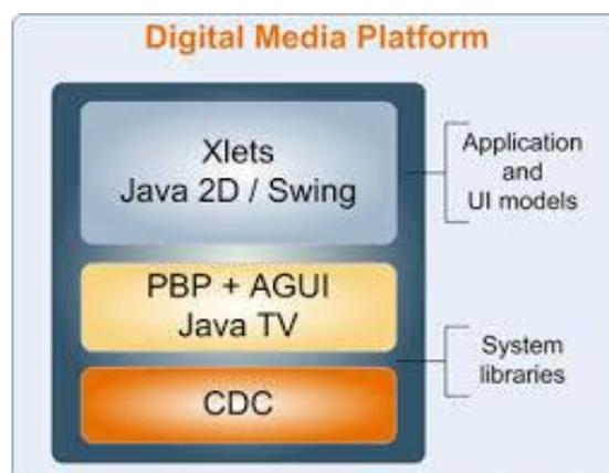
Figure C: The Connected Device Configuration (CDC)
