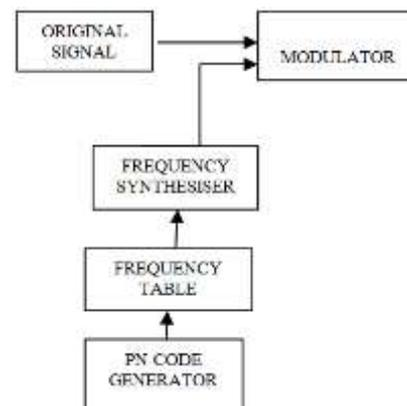
Figure 2. Block Diagram of FH Spectrum
