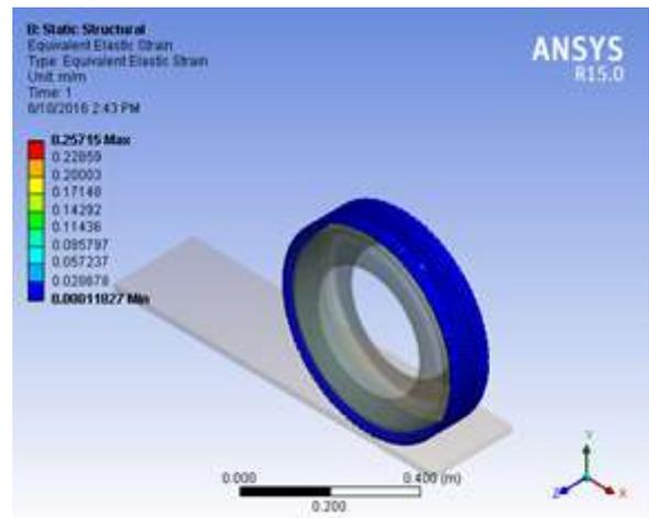
**Figure 7.** Equivalent Elastic Strain (m/m) in tread 2 (source CTAE CAD LAB)
