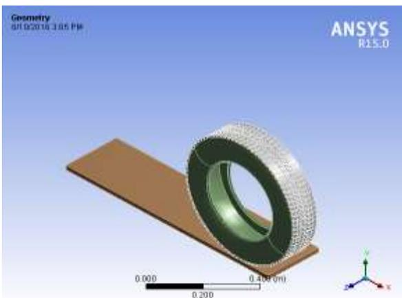
**Figure 3.** Analysis of tyre in Ansys
