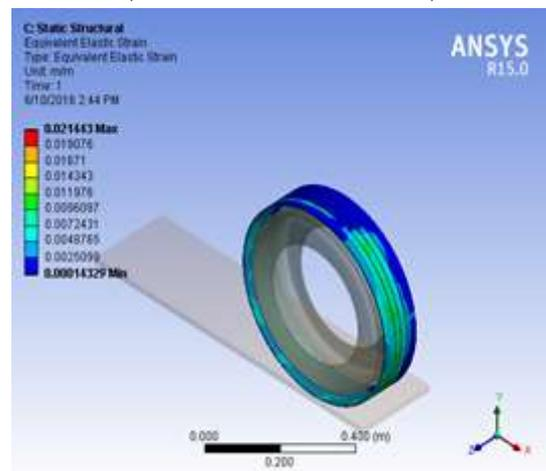
**Figure 8.** Equivalent Elastic Strain (m/m) in tread 3 (source CTAE CAD LAB)
