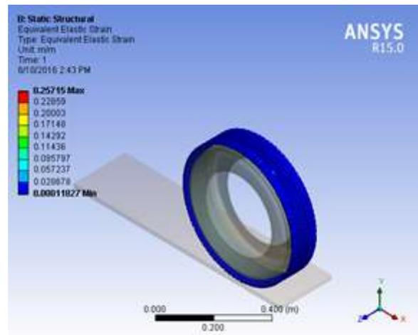
**Figure 7.** Equivalent Elastic Strain (m/m) in tread 2 (source CTAE CAD LAB)
