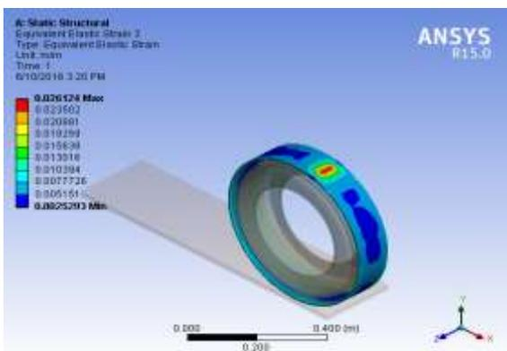
**Figure 6.** Equivalent Elastic Strain (m/m) in tread 1 (source CTAE CAD LAB)
