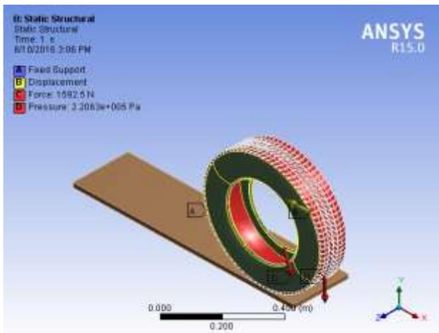
**Figure 5.** Pressure and Force diagram of tyre (Source: CAD lab CTAE)
