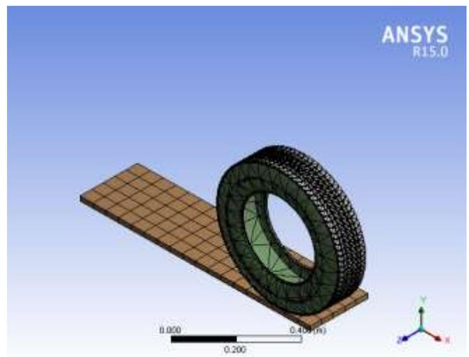
**Figure 4.** Meshing of Tyre (Source CTAE CAD Lab)
