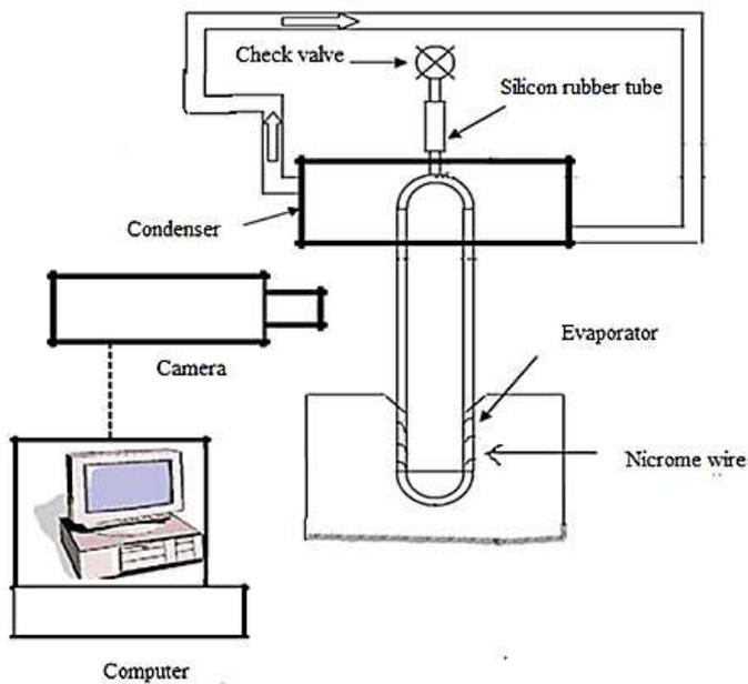
**Figure 3.** Experimental layout of CLPHP
