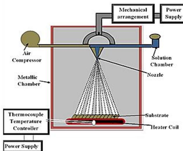
**Figure 1.** Systematic Diagram of Spray pyrolysis system
