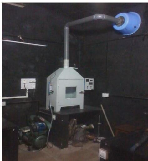
**Figure 2.** Photograph of Spray pyrolysis system.
