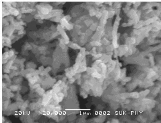
**Figure 7.** The SEM images of LSM thin films sintered at 650°C.
