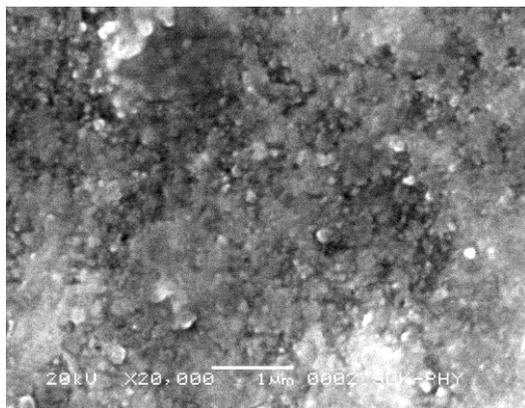
**Figure 6.** The SEM images of asprepared LSM film
