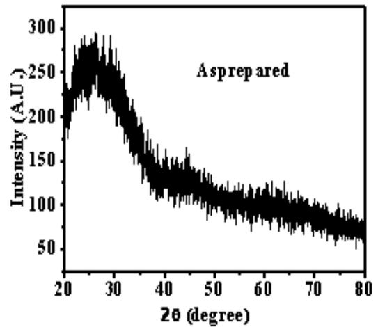
Figure 4. The XRD of LSM thin films asprepared
