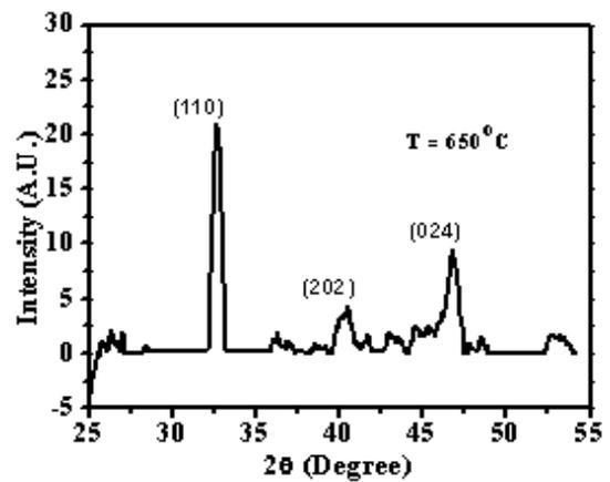
Figure 5. The XRD of LSM thin films sintered at  $650^\circ\text{C}$ .
