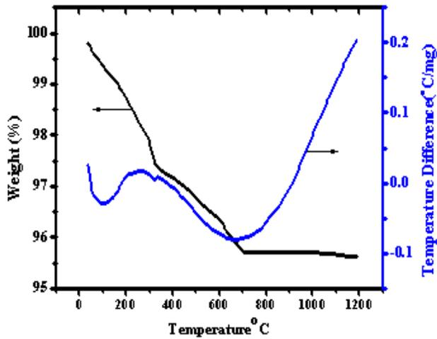
Figure 3. TG/DTA curve of LSM
