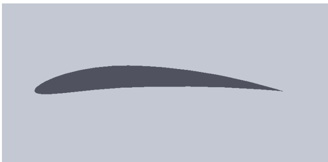
Figure 1. NACA- 6409 Airfoil Source- CAD LAB, CTAE
