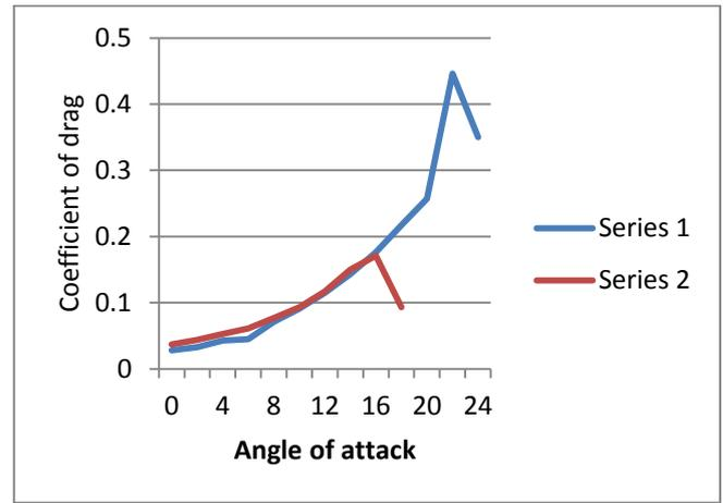
**Graph-2:** Coefficient of Drag for Airfoil section 1 and 2 vs. Angle of attack
