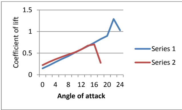
**Graph-1:** Coefficient of Lift for Airfoil section 1 and 2 vs. Angle of attack
