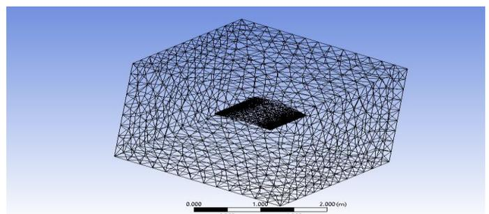
**Figure 3.** Mesh generation for airfoil Source - CAD LAB, CTAE
