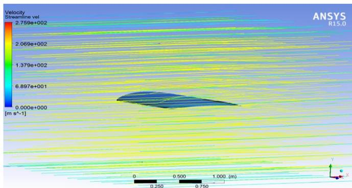
**Figure 4.** Velocity Streamline through an Airfoil 1
