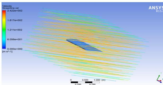
**Figure 5.** Velocity Streamline through Airfoil 2 Source
