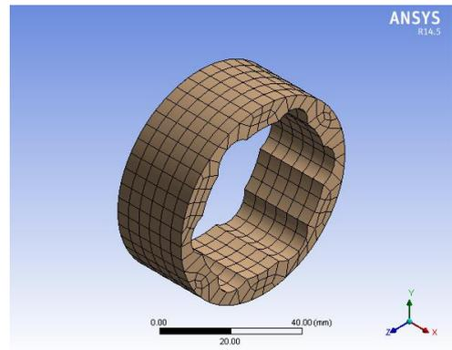
Figure 17. Meshing of Input Coupler Female Liner
