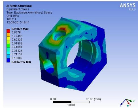
Figure 29. Von-Mises Stress of Trunion Holder
