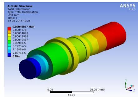
Figure 6. Total Deformation of Input shaft
