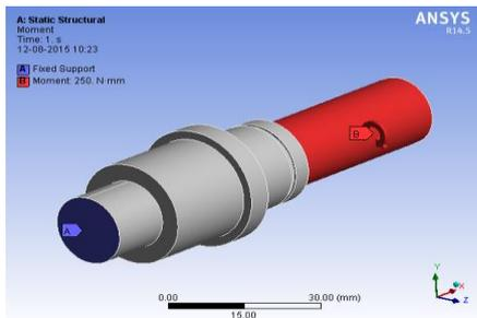
Figure 4. Static Structure of Input Shaft with Fixed Support & Moment
