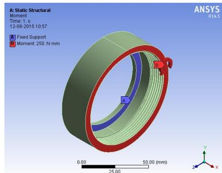
**Figure 13.** Static Structure of Input Coupler Ring with Fixed Support & Moment
