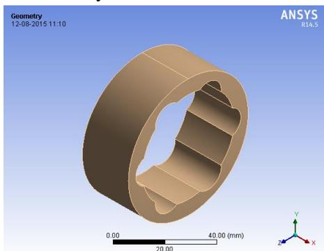
Figure 16. Geometry of Input Coupler Female Liner
