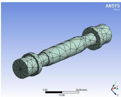
Figure 22. Meshing of Coupler Pin
