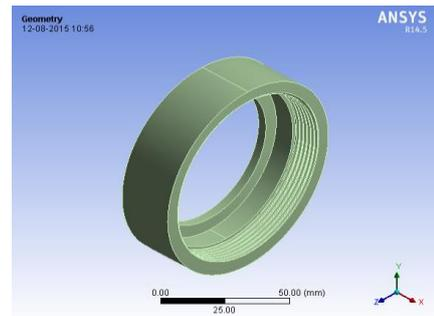
**Figure 12.** Modeling of Input Coupler Ring
