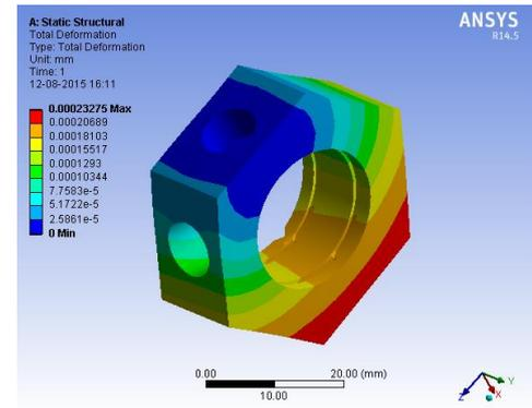
Figure 30. Total Deformation of Trunion Holder
