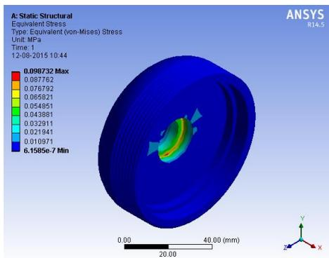
**Figure 10.** Von-mises stress of Input Coupler Body
