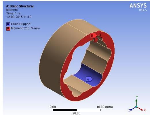
Figure 18. Static Structure of Input Coupler Female Liner with Fixed Support & Moment
