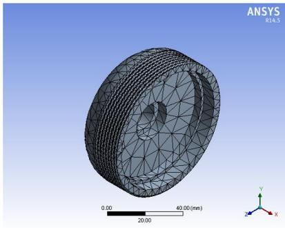
**Figure 8.** Meshing of Input Coupler Body
