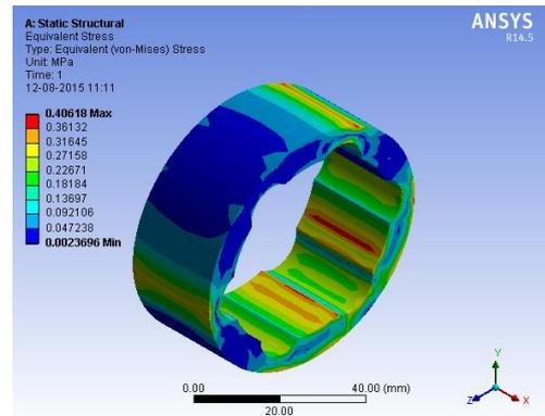
Figure 19. Von-Mises stress of Input Coupler Female Liner
