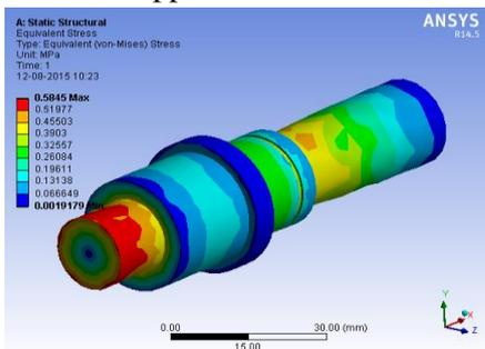
Figure 5. Von-Mises stress of Input Shaft
