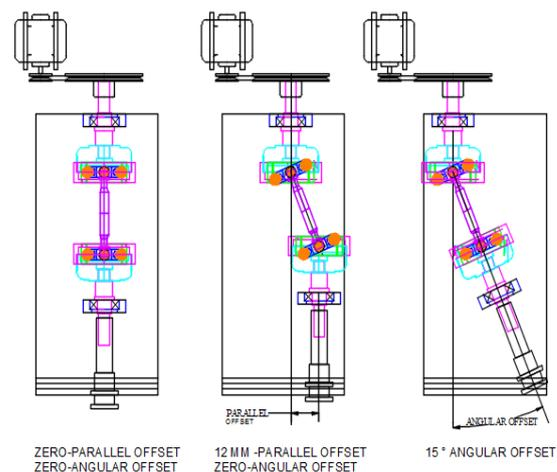
**Figure 1.** Arrangement of Test Rig
