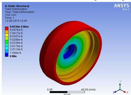
**Figure 11.** Total Deformation of Input Coupler Body
