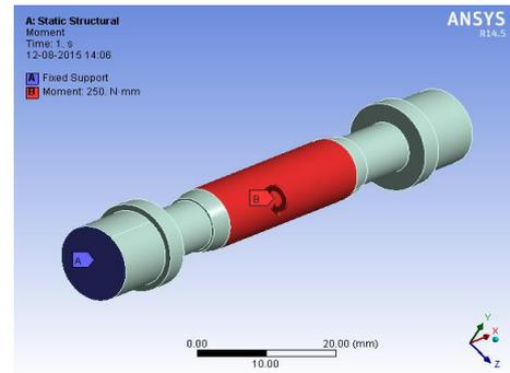
Figure 23. Static Structure of Coupler Pin with Fixed Support & Moment
