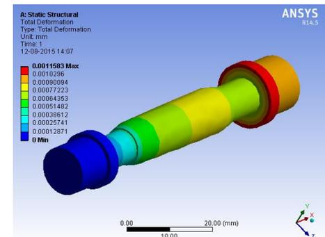
Figure 25. Total Deformation of Coupler Pin
