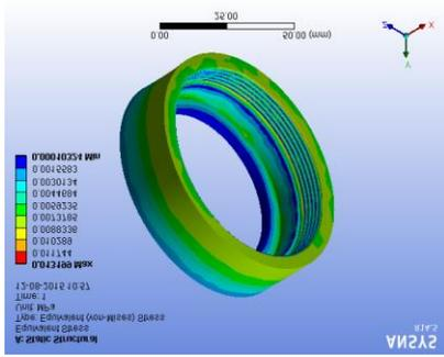
Figure 14. Von-Mises stress of Input Coupler Ring
