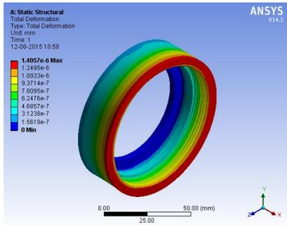
Figure 15. Total Deformation of Input Coupler Ring
