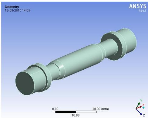
Figure 21. Modeling of Coupler Pin
