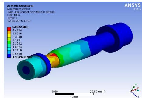
Figure 24. Von-Mises stress of Coupler Pin
