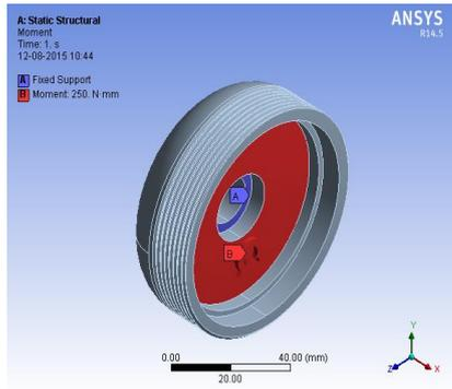
**Figure 9.** Static Structure of Input Coupler Body with Fixed Support & Moment
