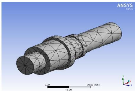
Figure 3. Meshing of Input Shaft
