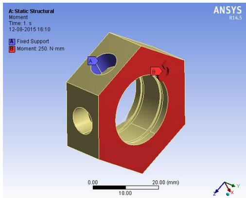
Figure 28. Static Structure of Trunion Holder with Fixed Support & Moment
