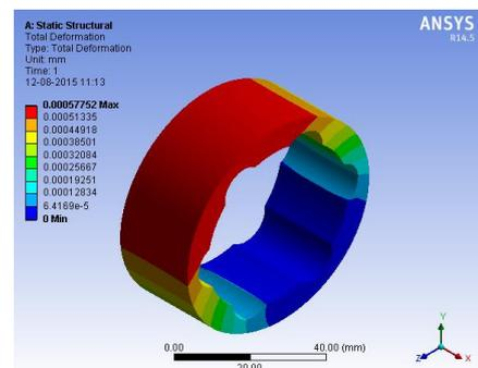
Figure 20. Total Deformation of Input Coupler Female Liner
