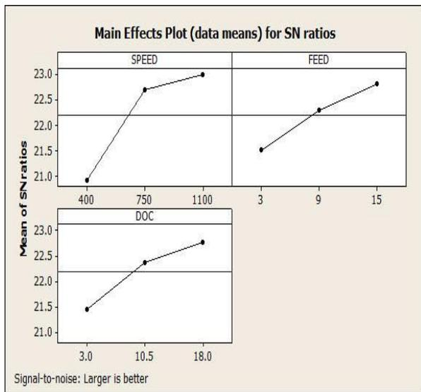
After conducting the experiment on surface grinding of austenitic stainless (AISI 321) surface finish are given below.
