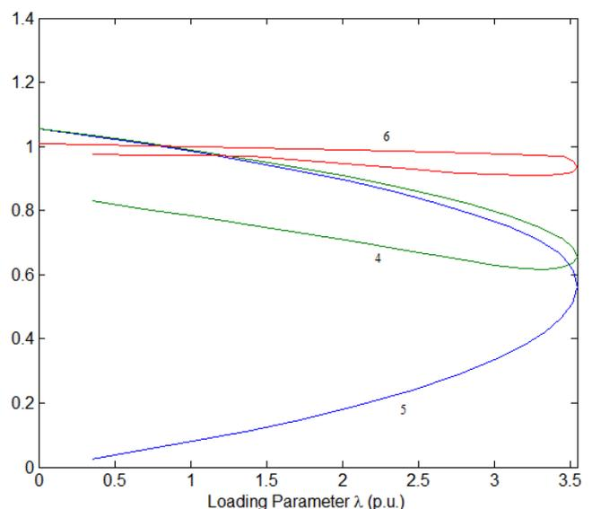
**Figure 4.** P-V Curves with STATCOM at Bus 6
